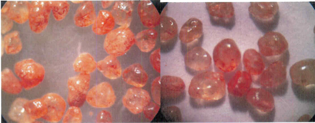
Figure 3: 30 min 2 (left) and 30 min 3 (right) after 5.200 cycles tread simulation.
